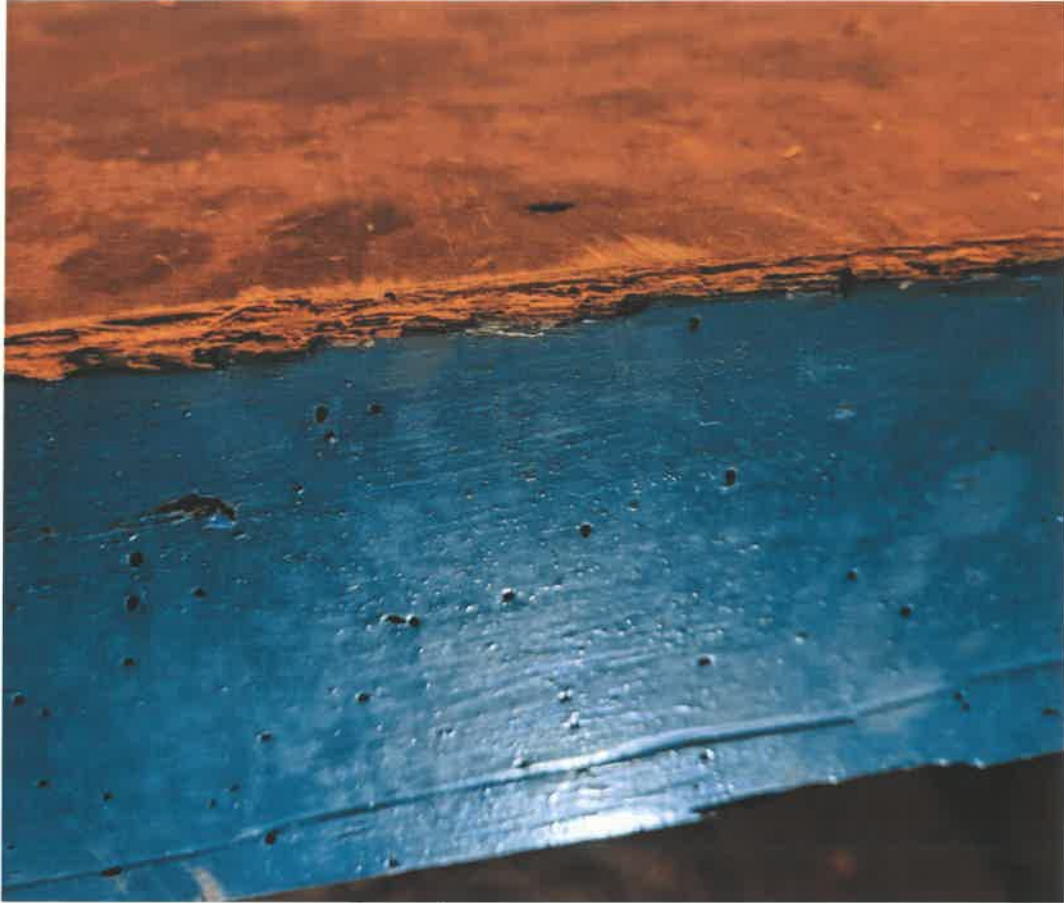
59 Woodworm to Clock Casing
